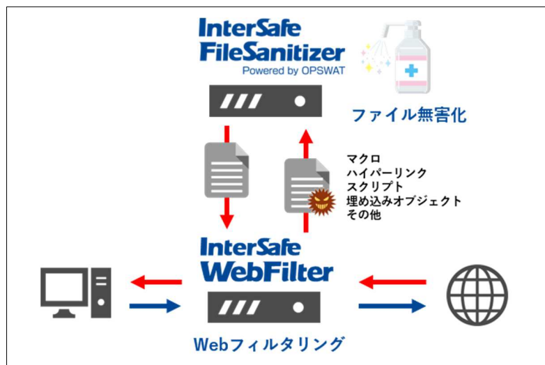
▲「InterSafe WebFilter」と「InterSafe FileSanitizer Powered by OPSWAT」の構成イメージ(Proxy 版)
