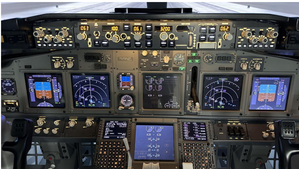
Figure 2.26 Physical diagram of the WB B737NG instrument panel
